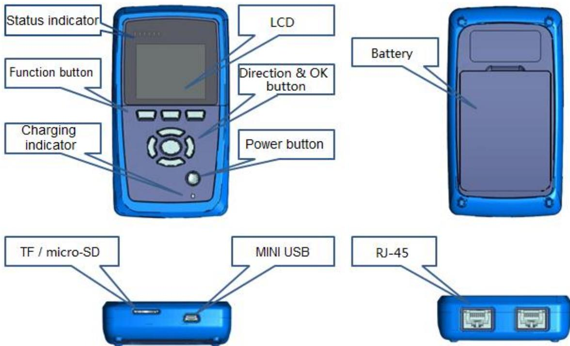
NL-830 has two RJ-45 ports on the top and has one Micro SD card connector, one Mini USB connector on the bottom. Front have six LED status indicator and one charging indicator. NL-830 has one 2.2 inch LCD screen, the battery install in the back.
